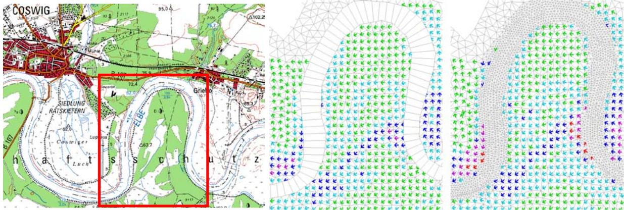
Figure 2: Comparison of calculated overflow near Coswig using a regular 2D model and the interlinked 1D/2D model.
