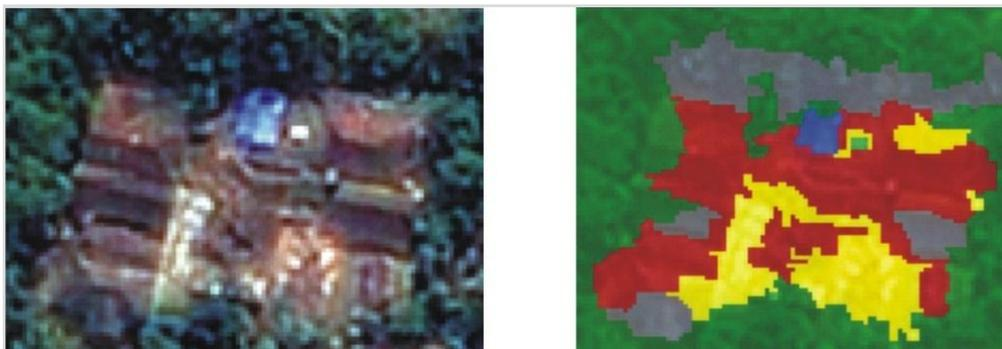
Figure 9: Rubble classified using object-oriented image classification; the colour code corresponds to the classes in figure 6.
