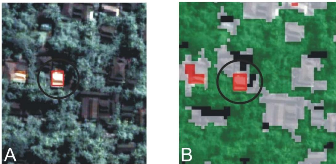
Figure 7: Segmentation and Classification applied on Quickbird imagery. Figure A shows an image object representing a single house. Figure B shows the same Image Object classified as a House with a red roof.
