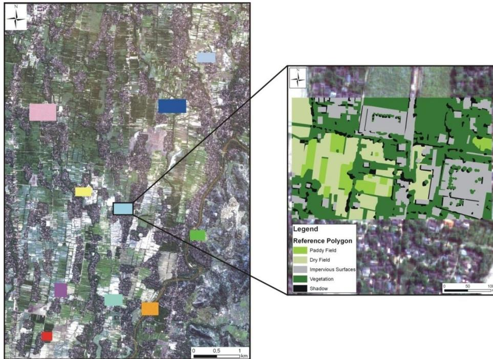
Figure 16: Location of reference data sets for object-oriented accuracy assessment and manually digitized classes from pre-event, panchromatic Quickbird Imagery acquired 2003.
