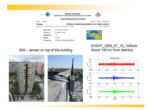
**Fig. 5**: Example of a SN deployed as part of the test network in the Ataköy district, Istanbul. Also shown are the recordings of a small event that occurred around 140 km from Istanbul.
