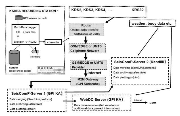
**Fig. 1**: Planned design of the KIMNET experiment (status Sept. 2008; subject to further changes). The seismological broadband recording stations KRS1-KRS32 will transmit the data via the cell phone network and internet to Karlsruhe. Other environmental data (weather, traffic etc.) will be added. Data dissemination is done via the WebDC tool.
