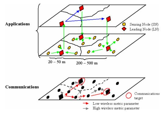
**Fig.1**: Layout of the Self Organising Seismic Early Warning Information Network based on groups of Sensing Nodes (yellow) which form clusters with a Leading Node. The Leading Nodes (red) decide on the detection validity and classification of seismic events.
