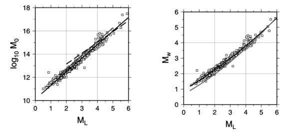
**Fig. 3**: (Left)  $\log_{10}M_0$  versus *Ml* (squares). Equation (2) from this study (black line), Grosser et al. (1998) (gray line), and Durukal and Çatalyürekli (2004) (dashed line). (Bottom) *Mw* versus *Ml* (squares). Equation (4) from this study (black line) and Stromeyer et al. (2004) (grey line).
