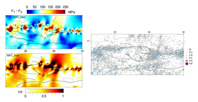
**Fig. 6**: Modelled differential stress  $\sigma_1 - \sigma_3$  at 5 km depth (left top) and calculated fracture potential (left bottom) in comparison to seismicity (right; 1973-1989 and 2005-August 2008 from USGS NEIC catalogue and 1990-2004 from Kandilli catalogue).
