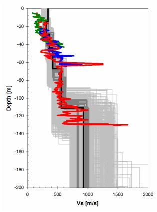
**Fig. 3**: Joint inversion results for Ataköy using the Picozzi and Albarello (2007) inversion scheme: all tested models (light grey), the minimum misfit model (black), models lying inside the minimum misfit  $\pm 10\%$  range (dark gray). Green, blue and red lines depict the PS logging results for the tests carried out in the 50,70, and 140 m deep boreholes, respectively.
