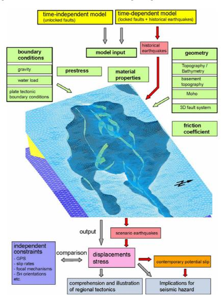
**Fig. 1**: Finite element mesh and modelling concept. The model incorporates the active fault system (yellow), topography and bathymetry (solid and transparent light blue, respectively), basement topography (dark grey) and the Moho (blue). Green boxes indicate the model input (geometry, boundary conditions, and material properties). Red arrows mark the additional work flow of the time-independent model with respect to the time-dependent one (grey arrows).
