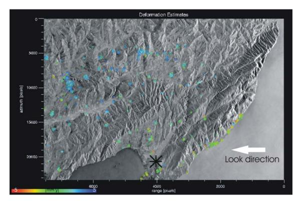
**Fig. 2**: Estimated line-of-sight (LOS) displacement rates at persistent scatterers across the Ganos fault between 1992 and 2000. The velocities are superimposed on the average amplitude SAR image. The black asterisk marks the reference point on the fault. Red corresponds to -5 mm/yr (LOS) motion away from the satellite and blue to 5 mm/yr (LOS) motion toward the satellite (Motagh et al., 2007).
