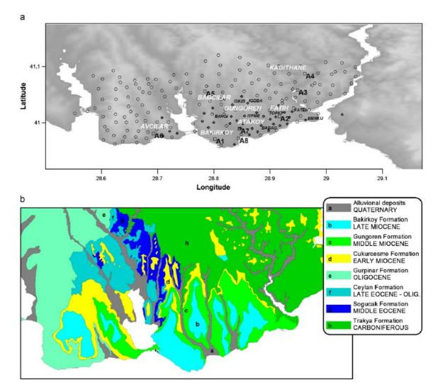
**Fig. 1**: Western part of Istanbul: (a) single station noise measurements at free field sites (dots), IERRS stations (rhombus, name of stations with earthquake recordings is indicated), and 2D array measurements (squares); (b) geological map.
